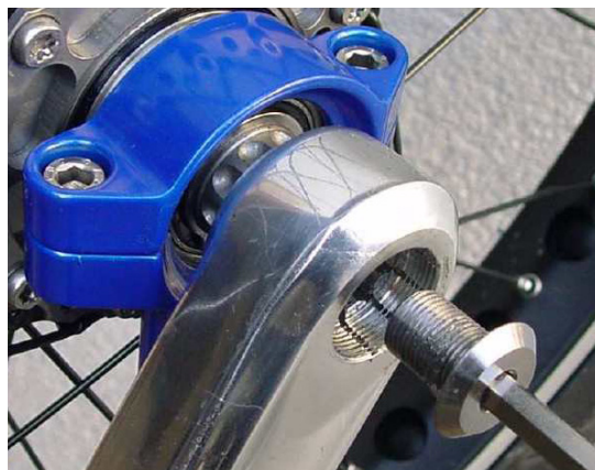
Picture 5: Mount crankarm and adjust axle bolt
