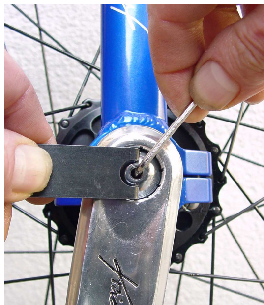
Picture 10: Loosen gear shift button
