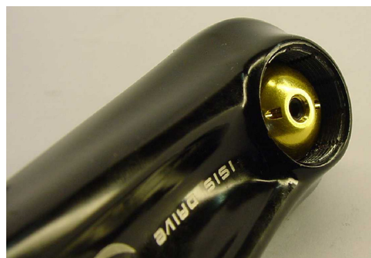
Picture 12: Check crankarm for sufficient space for gear shift button
