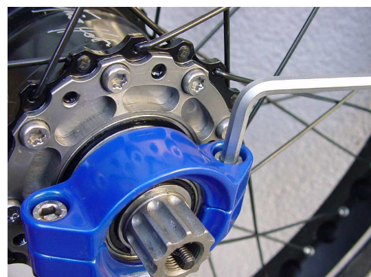
Picture 4: Tighten the screws evenly with 5-6 Nm!
