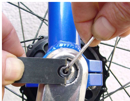
Picture 7: Hold the gear shift button with the black wrench and tighten it well with an 2.5 Allen wrench
